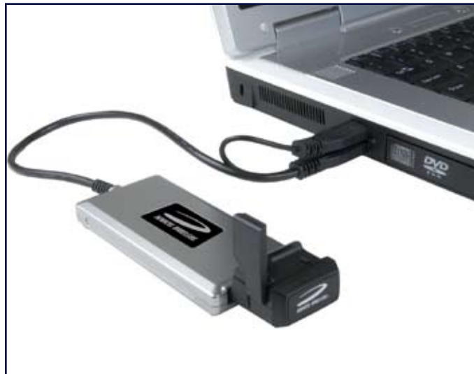
Second connector for extended RF performance
