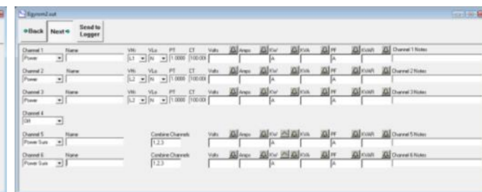
ELOG Setup Dialog Box 2: Configure your logger to meet your metering needs.
