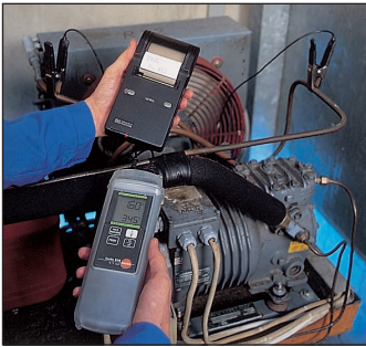
Determines refrigeration unit efficiency with printout of readings on location
