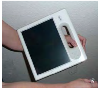
Rest the C5 on your forearm and pass medication in front of bar code reader
