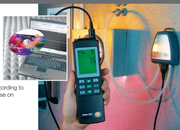
Monitors filters using the external 100 Pa probe
