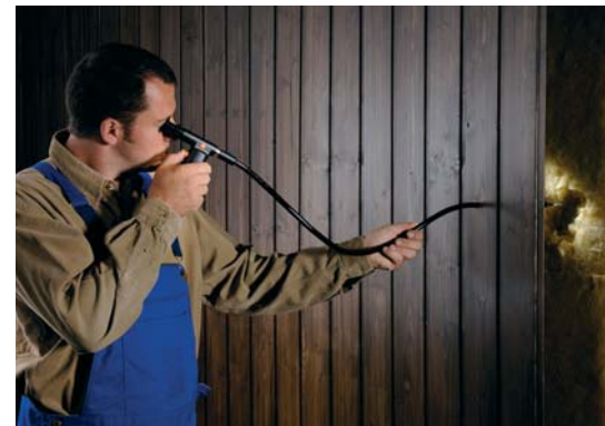
Checks insulations by using the stability of the Decabon tube
