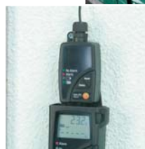
Alarm message, reliable notification when limits are exceeded
