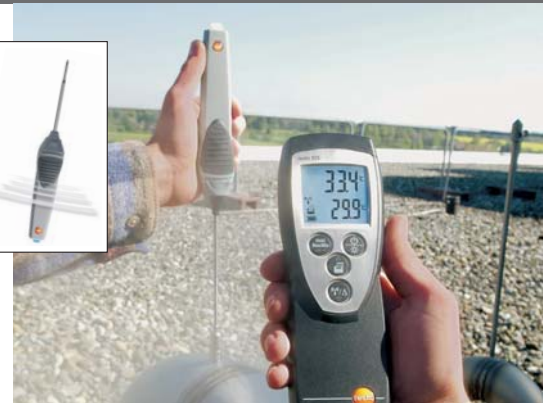
Monitoring temperature at exhaust outlets
