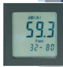
Frequency weighting of current reading Time weighting Section measurement range
