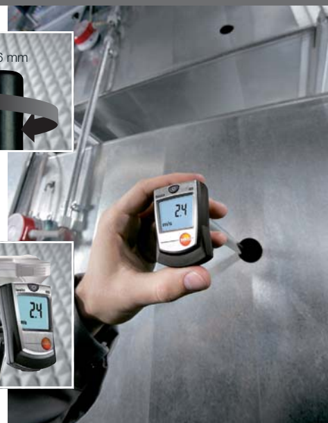
Ideal for measurements in ducts
