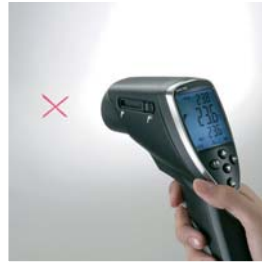
Switch optics 1: Far-field 75:1 (16 mm, distance 1200 mm) with cross laser sighting
