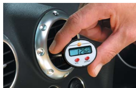
Measurements on air conditioning units
