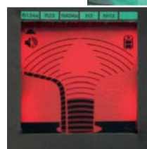
Maximum indicator shows maximum leakages
