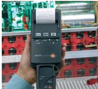
Fast printout and logger rebooting with testo 575
