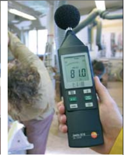
testo 816, Checking noise control
