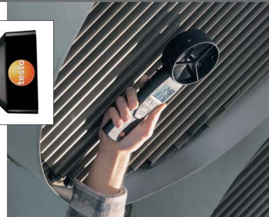
Measuring exhaust air with testo 417 and built-in 100 mm Ø vane
