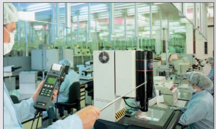
Checking flow speed using the hot wire probe Part no.: 0635 1047
