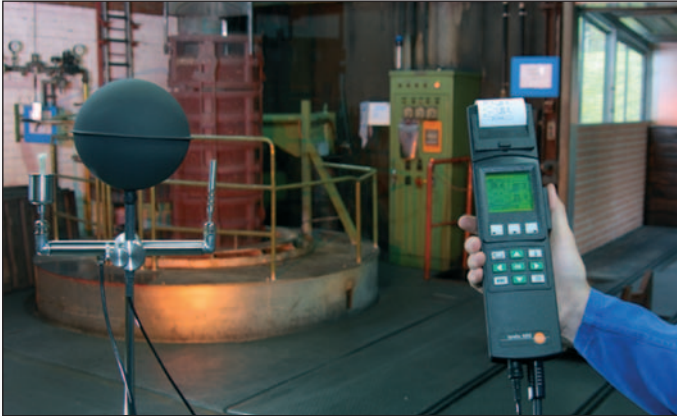
Measure with testo 400 and WBGT probe
