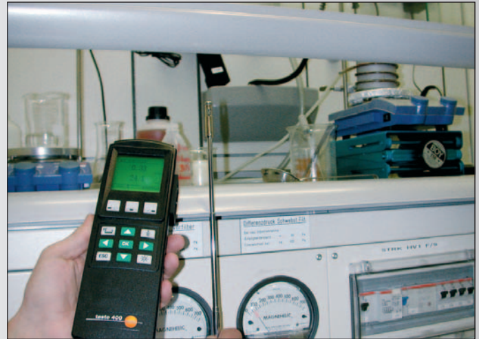
On-site testing of a laboratory fume cupboard with testo 400
