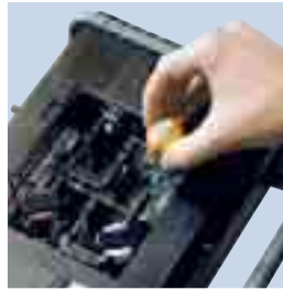
Gas sensors can be changed quickly and easily by the user on site
