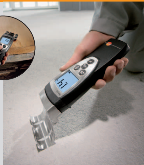
Fast and easy – moisture checks on screed. Measuring several points across a surface ensures more security.
