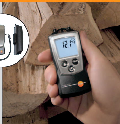
Checking wood moisture
