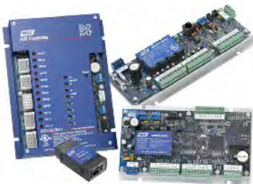
Figure 1: Building control systems by ASI Controls monitor and control energy consumption at Safeguard's storage locations.
