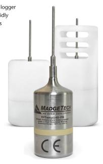
The Trigger Settings feature of the HiTemp140-FR allows users to configure high and low temperature thresholds that when met or exceeded, will automatically start or stop recording data to memory. This data logger is capable of storing up to 32,700 date and time stamped readings and features a nonvolatile solid state memory which retains data even if the battery becomes discharged.
