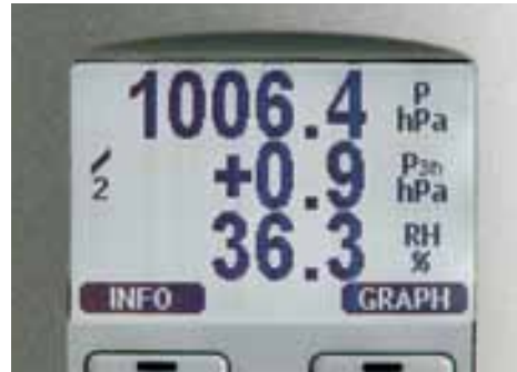
The display also shows the WMO pressure trend \Delta P 3h and tendency of 0 ... 9.
