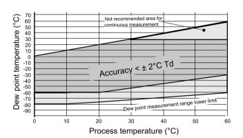
DEW POINT ACCURACY VS. MEASUREMENT CONDITIONS
