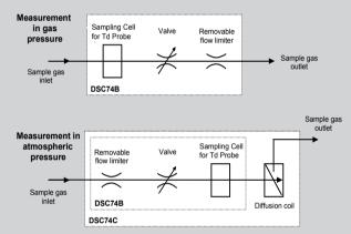
The DSC74B sampling cell enables the measurement of the sampled gas either in gas pressure up to 10 bar or in atmospheric pressure depending on the gas inlet and outlet. The DSC74C is like the DSC74B but with an additional coil to avoid back diffusion, the effect of surrounding moisture, in dewpoint measurements in atmospheric pressure.
