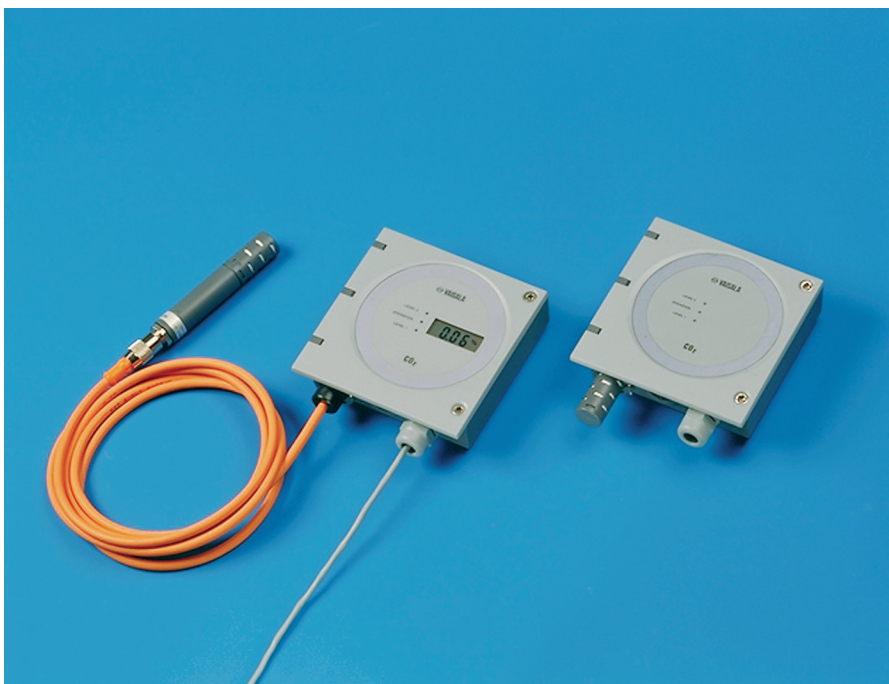
The GMT220 transmitters withstand harsh and humid environments.
