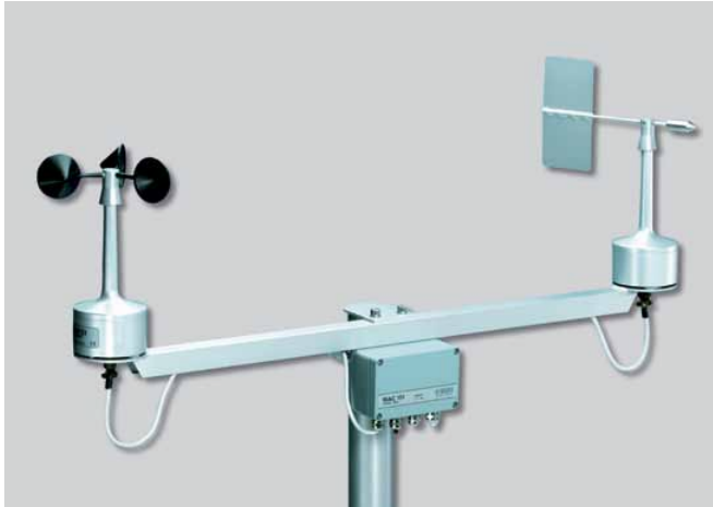
The WA15 is based on accurate sensors installed on a large crossarm. It is designed for demanding wind measurement applications.
