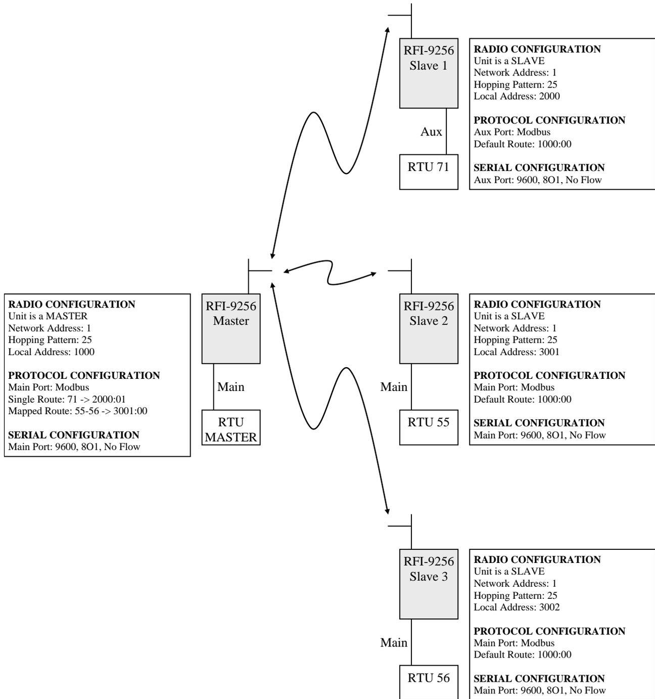
Figure 22: SCADA network with routing table
