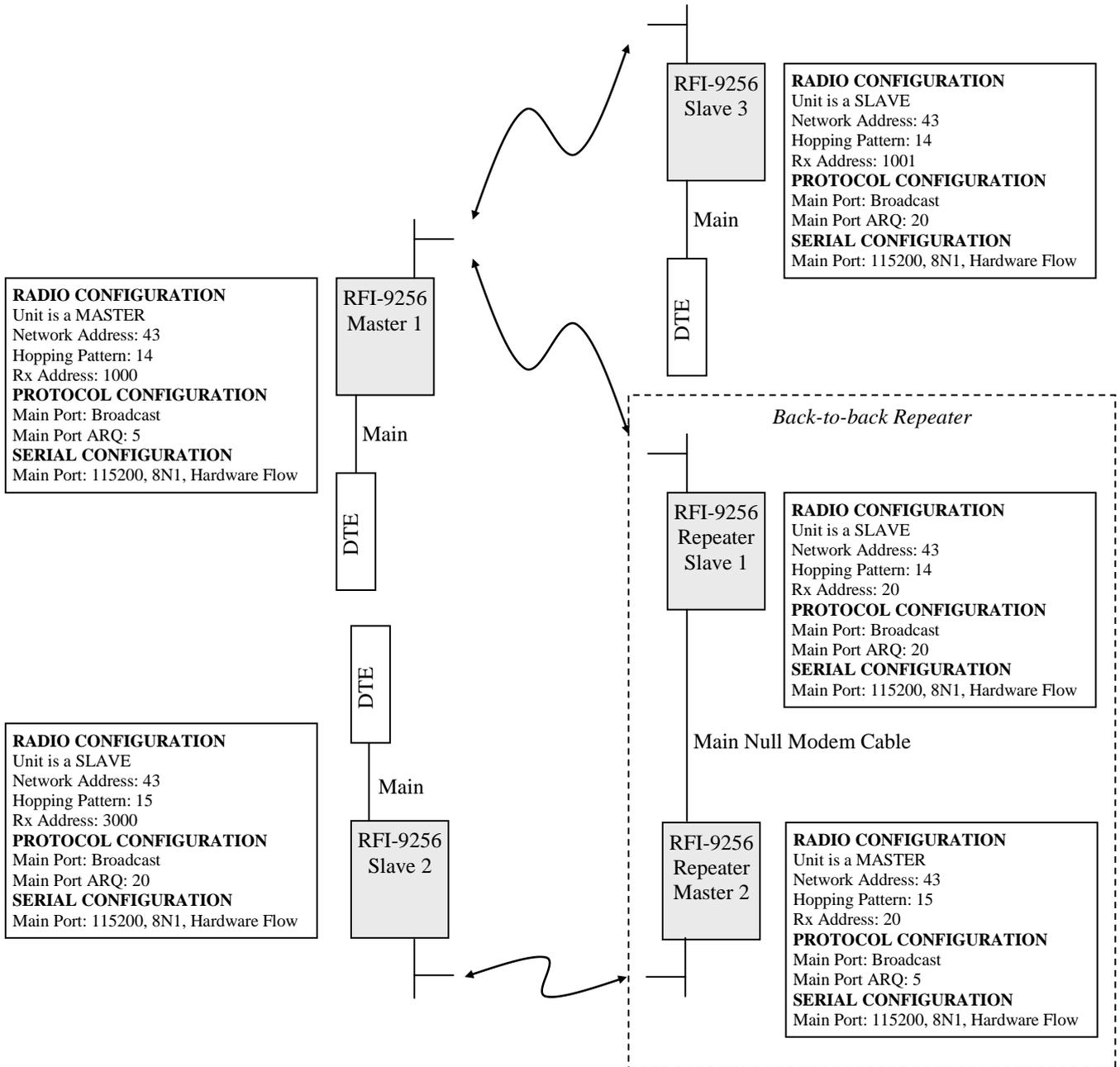
Figure 19: Point-to-multipoint broadcast network with three destinations and a back-to-back repeater
