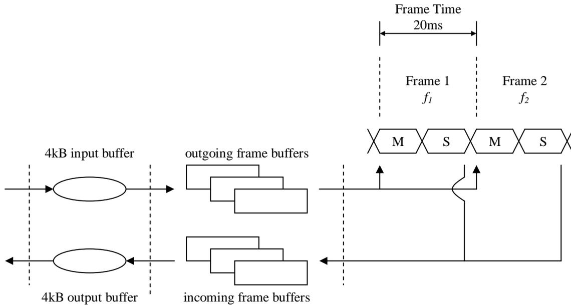
Figure 8: Overall data path in the RFI-9256 radio
