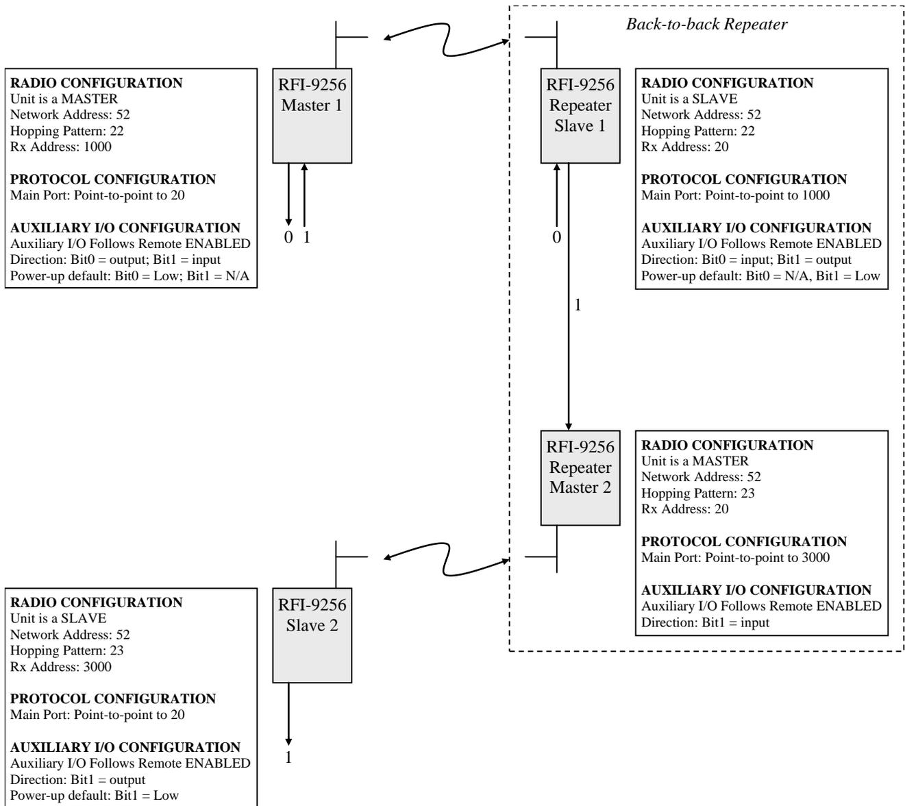
Figure 25: Point-to-point auxiliary I/O with a back-to-back repeater
