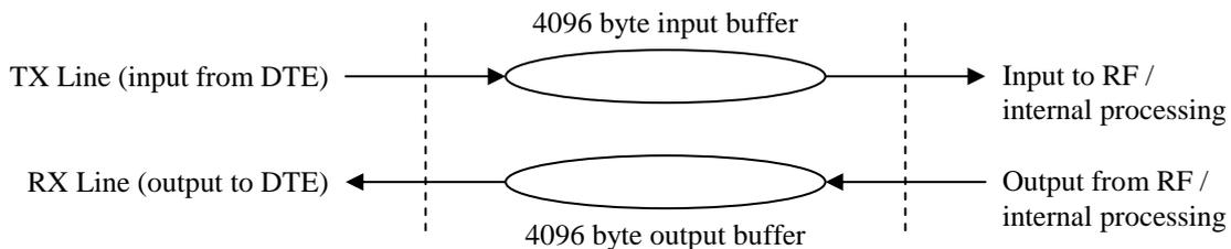
*Figure 6: Buffering scheme on the RFI-9256*
