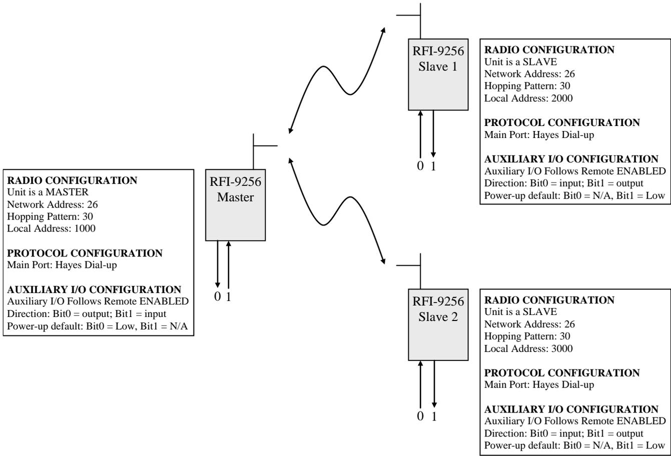
*Figure 26: Hayes Dial-up auxiliary I/O*
