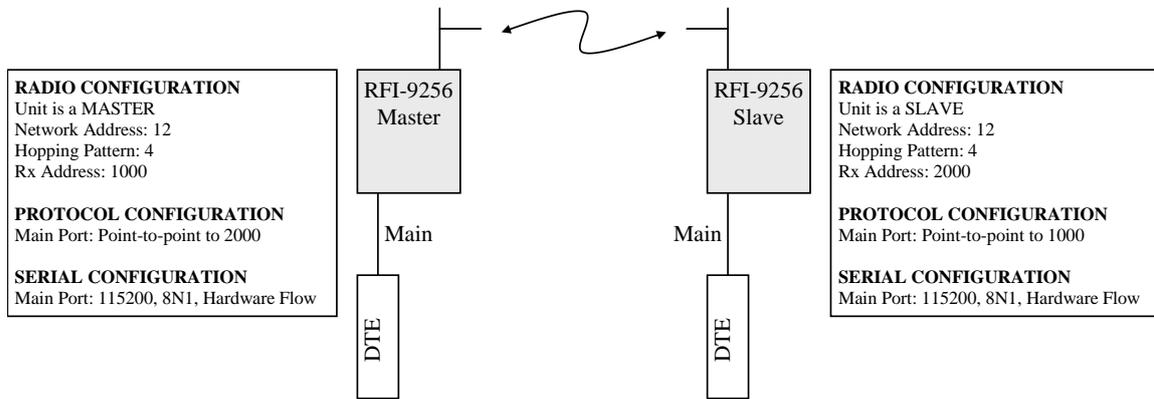
Figure 14: Basic point-to-point network
