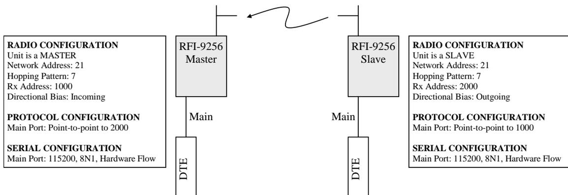
*Figure 15: Simplex point-to-point network*
