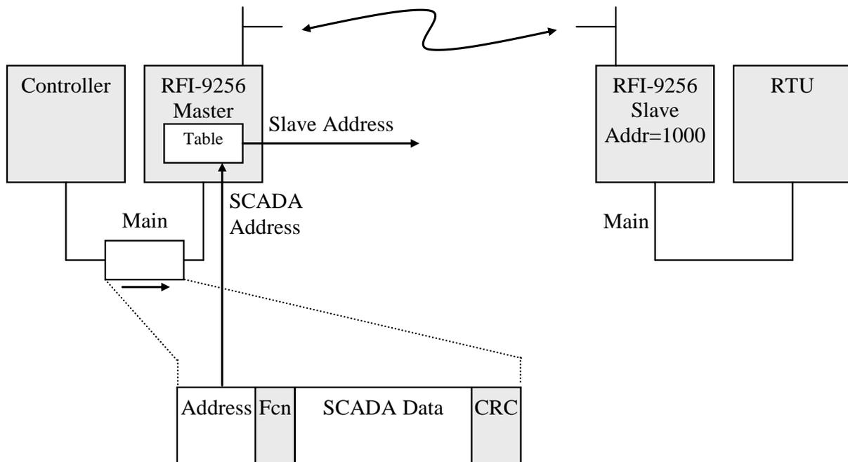
Figure 12: SCADA protocol routing
