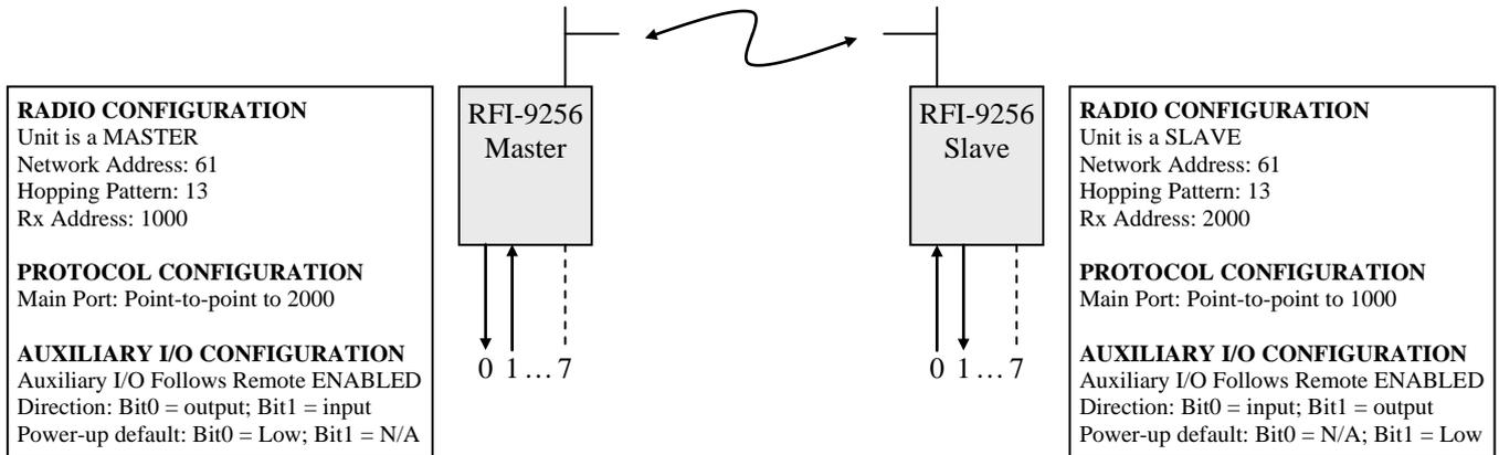
*Figure 24: Point-to-point routing of auxiliary I/Os*
