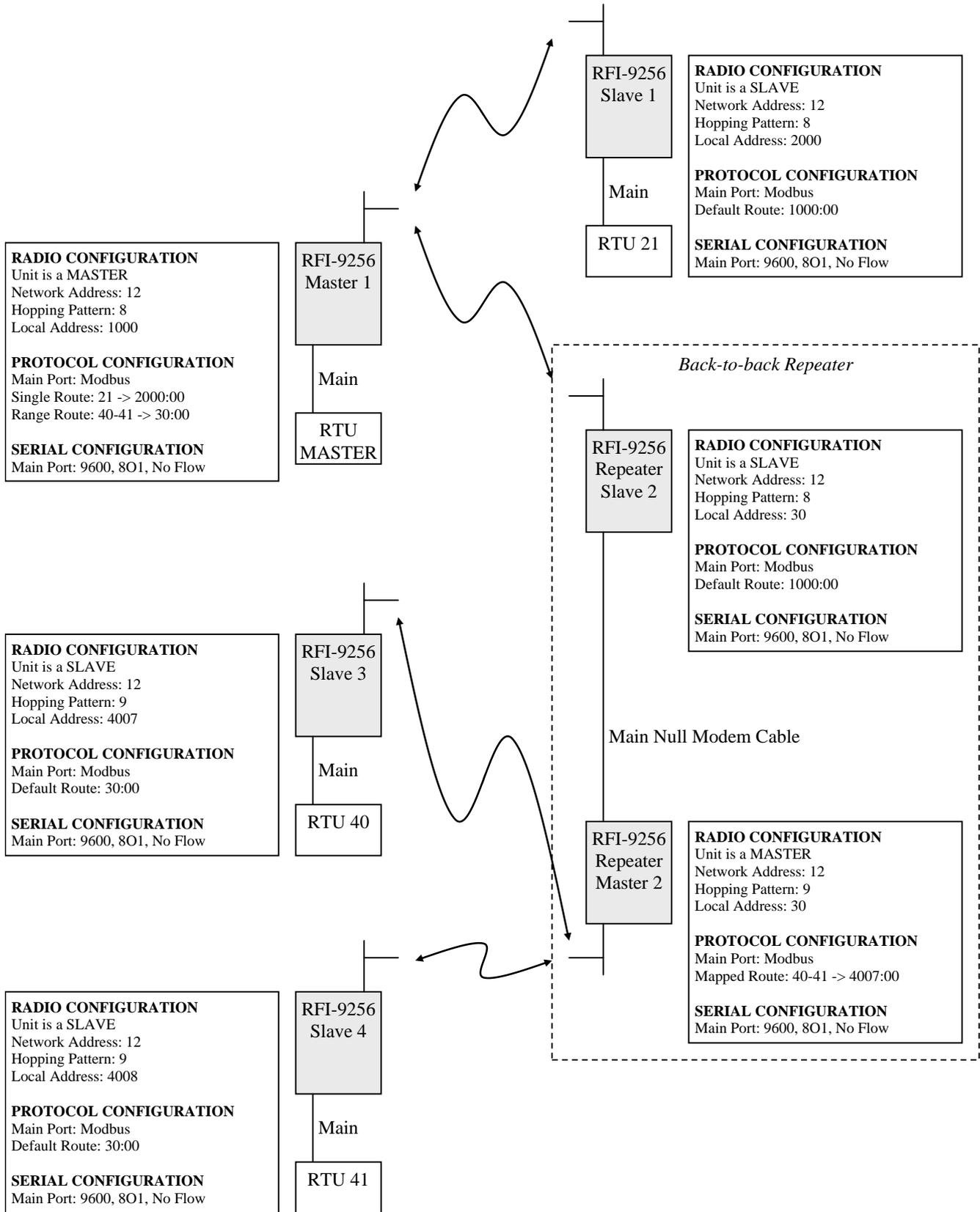
Figure 23: SCADA network with a back-to-back repeater
