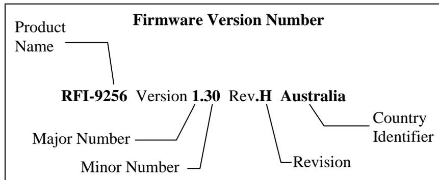
*Figure 30: Example firmware version number*
