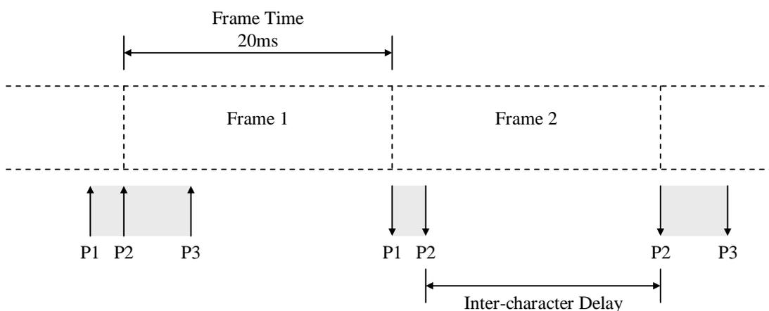
Figure 10: Data timing variation due to framing
