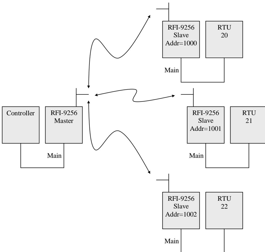
Figure 13: Range routing relationship between radio address and RTU address
