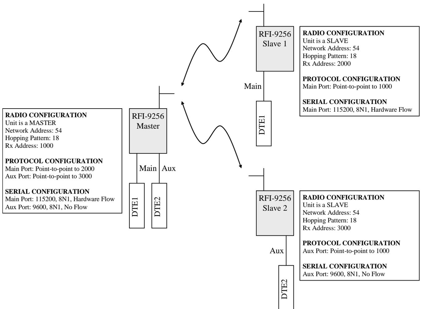
*Figure 16: Multiple slave point-to-point network*
