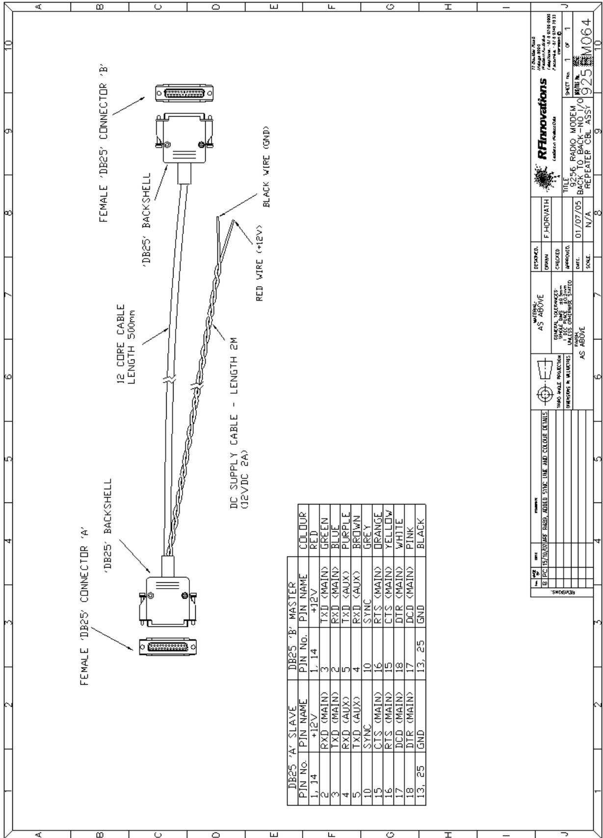
Figure 28: RFI-9256 back-to-back repeater cable assembly
