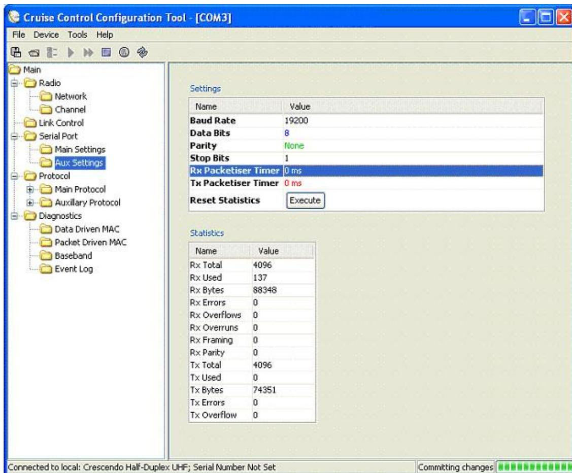
Figure 4: Cruise control configuration tool
