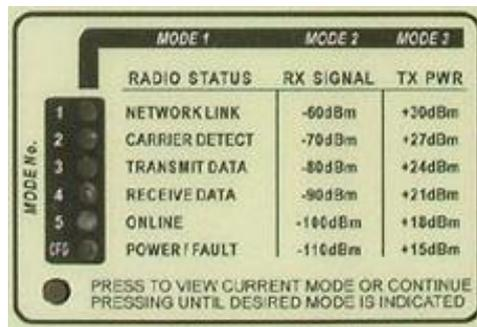
Figure 5: RFI-9256 front panel
