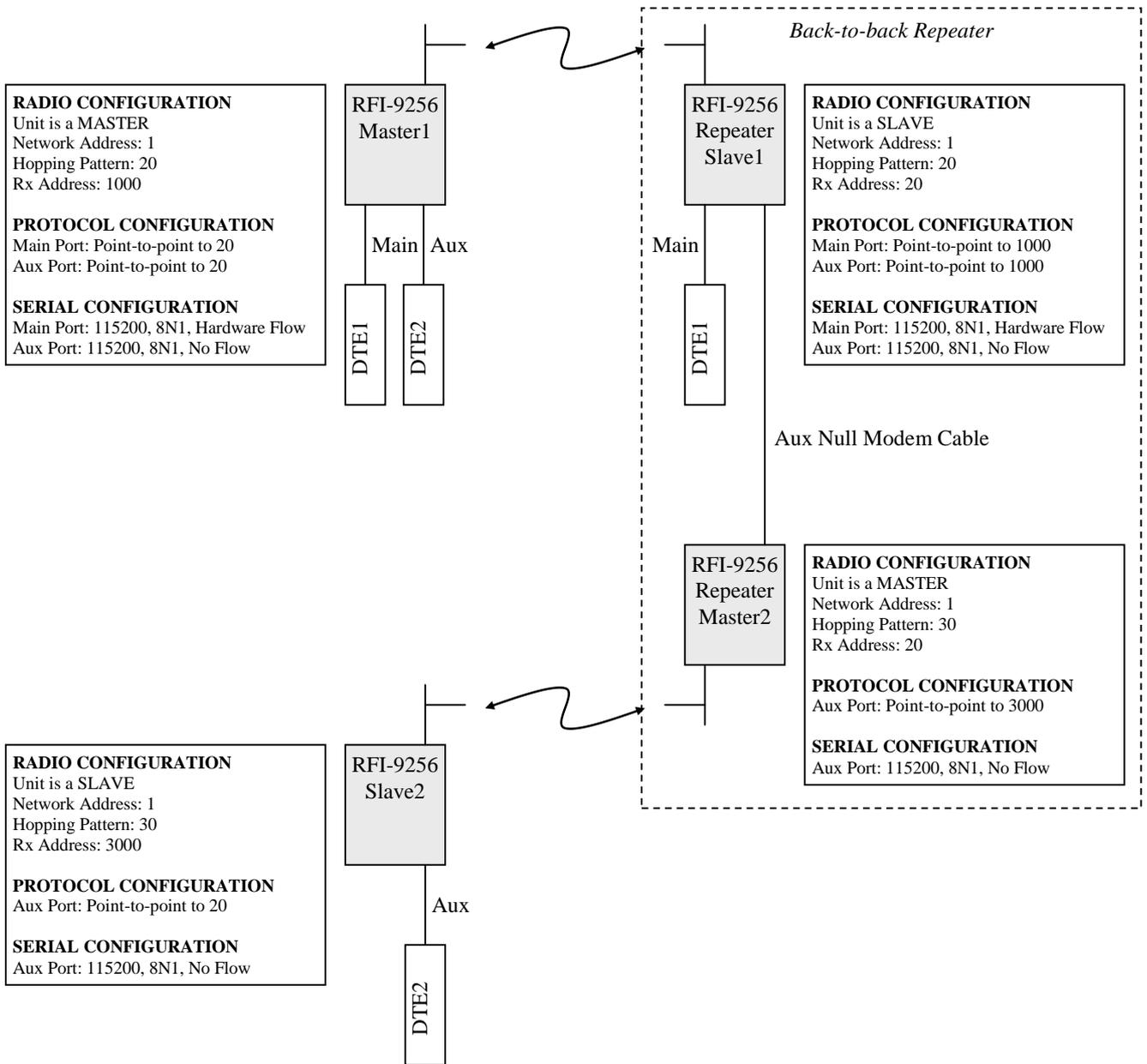
Figure 17: Point-to-point network with a back-to-back repeater
