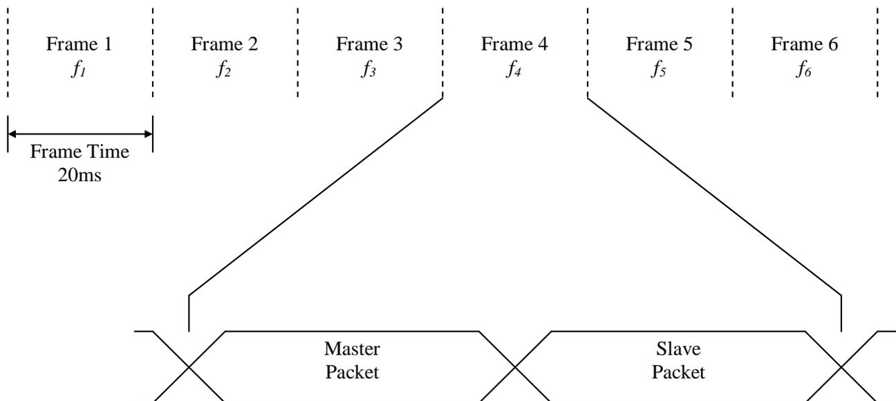
*Figure 7: RFI-9256 time division duplex / frequency division duplex (TDD/FDD) operation*
