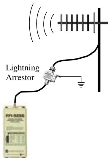
*Figure 1: Antenna connection*
