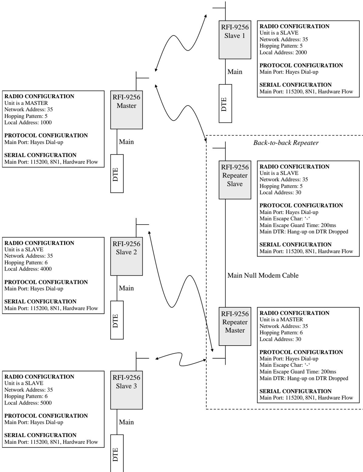
Figure 21: Hayes dial-up network with three destinations and a back-to-back repeater
