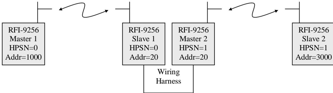
Figure 11: Back-to-back repeater configuration
