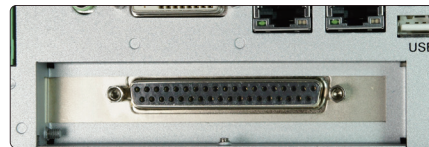
Full Height PCI or PCI-E Slot Opening
