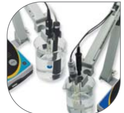
Integrated electrode holder – can be used on either side
