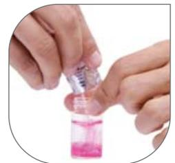
**Step 2:** Add reagent into sample vial (according to the specified parameter test procedure). Secure vial in meter sample well
