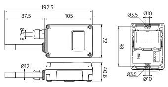
HMD82/83(D) and TMD82/83 RH+T and T-only transmitters for ducts
