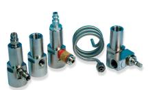
The sampling cells (from the left) DMT242SC2, DMT242SC and DSC74 can be used to connect the DM70 to sample gas flow. The DSC74B (right) is a two-pressure sampling cell that can be used for measurements in either pressurized or ambient pressure. The cooling/venting coil is included in the DSC74C sample cell, but is an option for all sampling cells.
