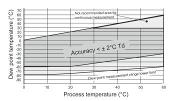
DEW POINT ACCURACY VS. MEASUREMENT CONDITIONS
