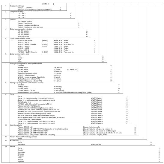
For freezing conditions select appropriate combination of heating and temperature ranges
