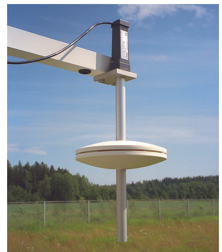
PTB210 paired with SPH10 static pressure head
