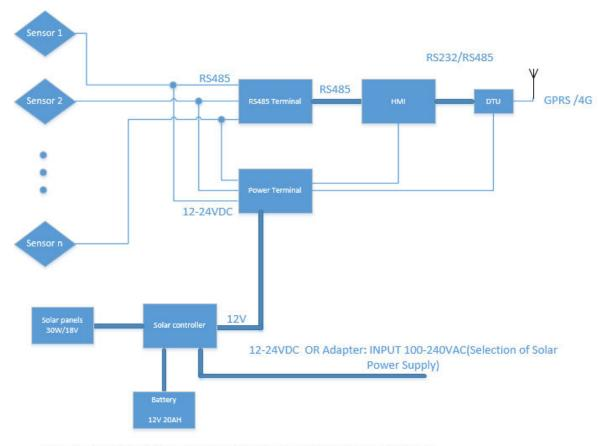
Note: Lead-acid batteries and lithium batteries use different solar controllers
